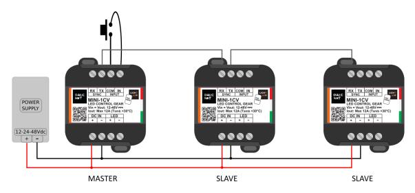
DEVICE SYNCHRONIZATION, ONE POWER SUPPLY FOR EACH DIMMER
